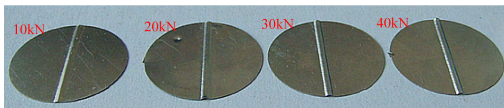
Fig. 6. Parts formed with different forming loads.
